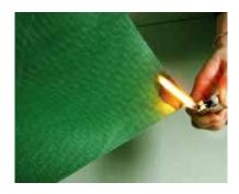
FRC-10/60 conforms to the requirement of LEED IEQ 4.2, NFPA Class A and IBC Class A
